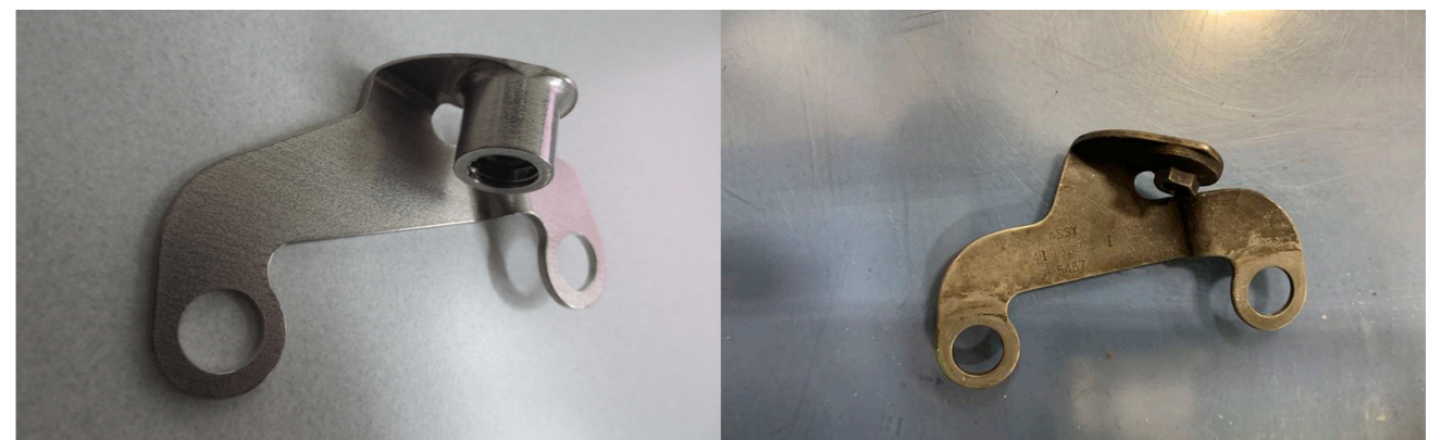
Legend: On the right, part made with a conventional manufacturing process; on the left, part made with an AM process. Credit: Pratt & Whitney
