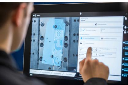
Maximize efficiency and save on material costs by printing directly on preform blanks, with precise geometry placement using our HMI and perfect alignment ensured by our advanced powder bed camera. Choose from sustainable reprocessing or high-volume series production to achieve high-quality results every time.
