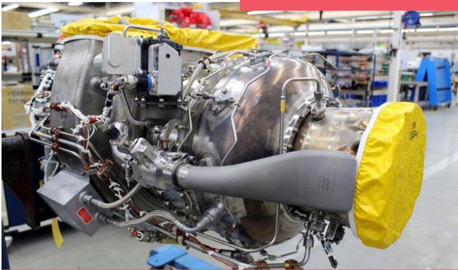
Courtesy of Honeywell Aerospace. RE220 commercial APU with the additive exhaust duct front and Center.
