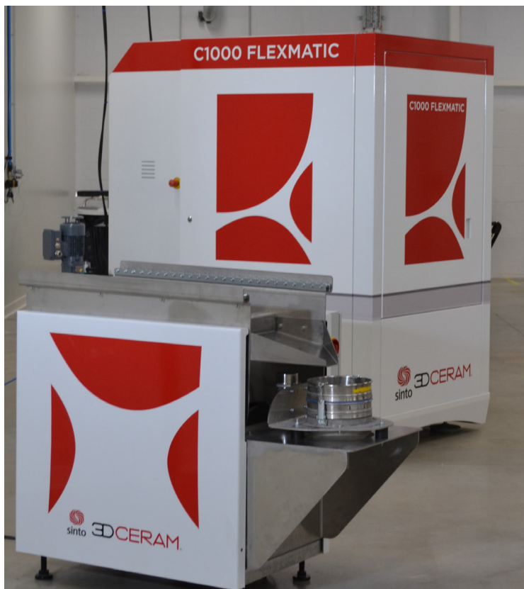
Fig 1. C1000 FLEXMATIC 3D printer and the recycling station work in an automatic line
