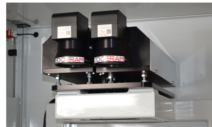
Fig 2. Two lasers increase productivity on C1000 FLEXMATIC. Courtesy of 3DCeram
