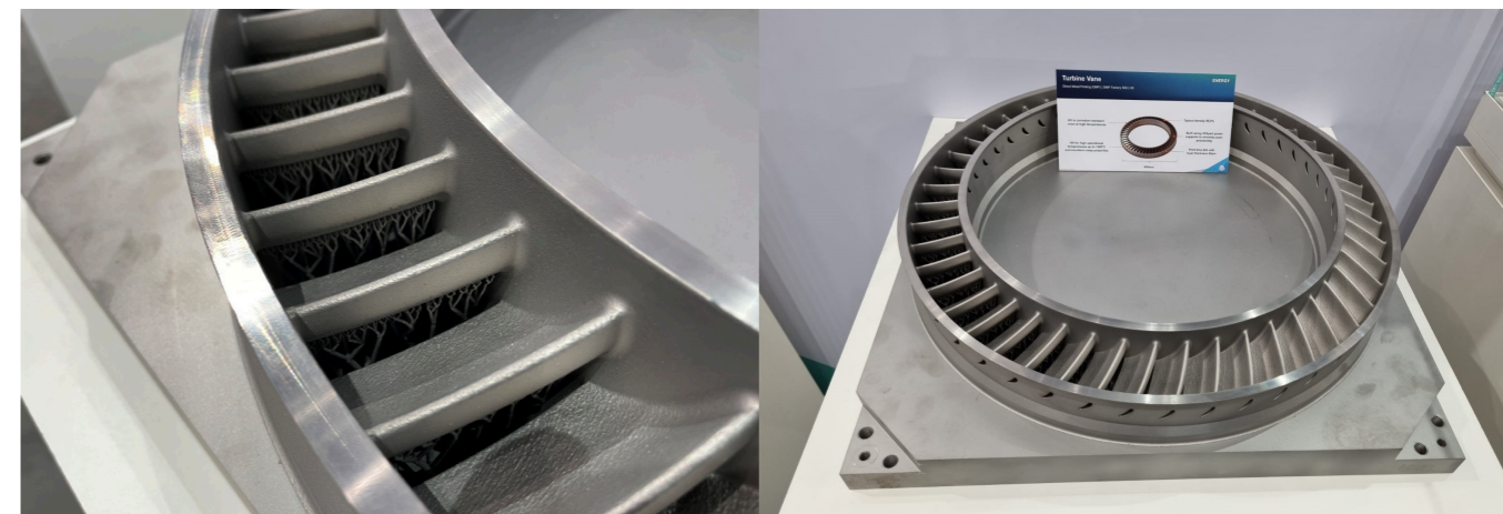
Turbine vane produced using breakaway supports. Credit: 3D Adept. Images taken on 3D Systems' booth at Formnext 2022.
