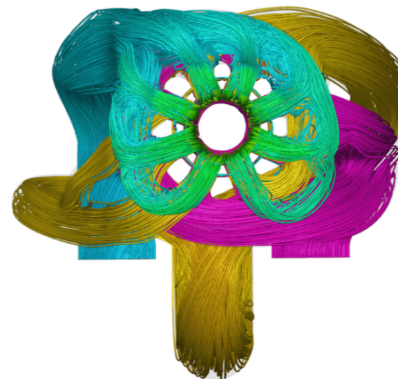
The image above shows fluid streamlines in a static Computational Fluid Dynamics model of a valve body. Credit: Domin.
