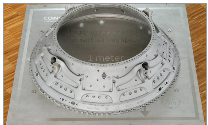
Legend: For this MOnACO project - a clean aviation experiment - the number of parts in an assembly has been reduced from more than 100 down to a single part. (Fusion 360 generative design was used in the structural and fluid flow design optimization for this project).
