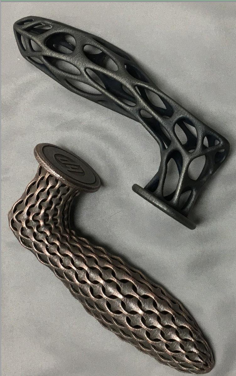
SAMPE Strength Comparison of Topology Optimized Lattice From Printed SLA Resin, Electroplated Resin and PBF Al – Courtesy of RePliiForm Inc.
