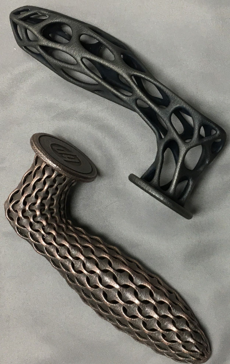
SAMPE Strength Comparison of Topology Optimized Lattice From Printed SLA Resin, Electroplated Resin and PBF Al – Courtesy of RePliForm Inc.
