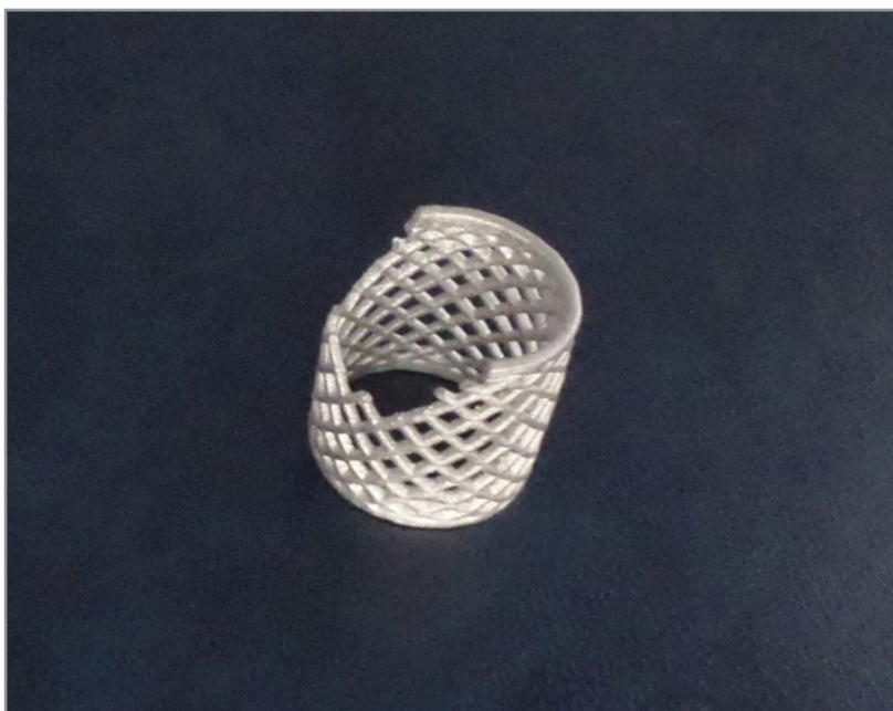
Sintered part, broken during depowdering due to low green part strength. Image via Fraunhofer IFAM.
