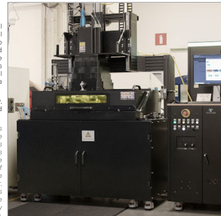
Legend: the image shows an Aerosint machine alongside an Aconity3D system, Aconity MIDI+. Today the multi-material printing approach was validated within a Laser Powder Bed Fusion process. The Aconity MIDI+ printer equipped with Aerosint's recoater is the first commercially available multi-material Laser Powder Bed Fusion printer in the world. Image: Courtesy of Aerosint.
