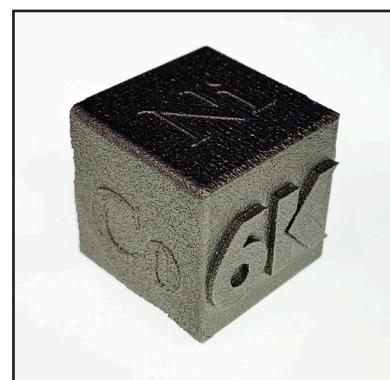
First 3D printed High Entropy Alloy part – Image: 6K
