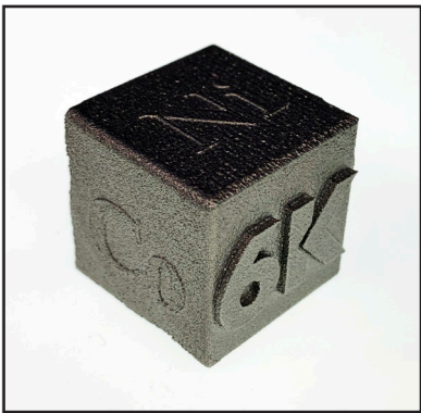
First 3D printed High Entropy Alloy part – Image: 6K
