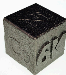
First 3D printed High Entropy Alloy part – Image: 6K
