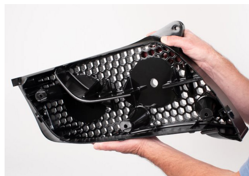
TOYOTA Gazoo Racing manufactured this automotive grill CNC fixture using 3D Systems' new Accura AMX Rigid Black – Image: 3D Systems.
