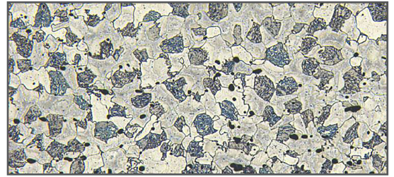
Legend: The cross-section of the FSLA material shows the dual-phase microstructure after heat treatment. Image: GKN Aerospace
