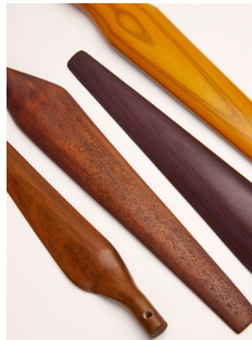
Image: The Forust process combines two waste streams from traditional wood production, sawdust and lignin, to sustainably produce isotropic, high-strength, wood parts. Courtesy: Desktop Metal
