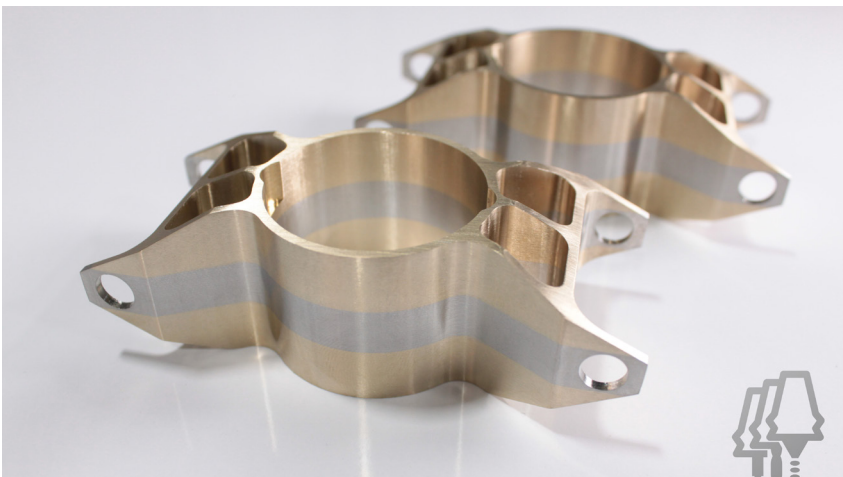
Image: Hybrid Manufacturing Technologies. Legend: Multi-metal brackets benefiting from the heat dissipation and lubricity of bronze with the strength of stainless steel, printed and finished in a hybrid CNC featuring the AMBIT™ FLEX system.
