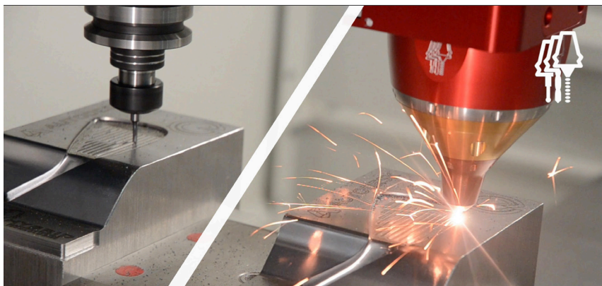
Credit: Hybrid Manufacturing Technologies – Legend: Tool steel forging die enhanced and finished in a single setup using a hybrid CNC featuring the AMBIT™ ONE LMD system
