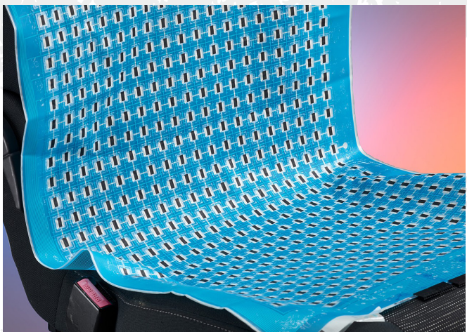
Image: Holst Centre – Together with the automotive industry, Holst Centre develops non-contact sensing solutions based on printed electronics technologies.
