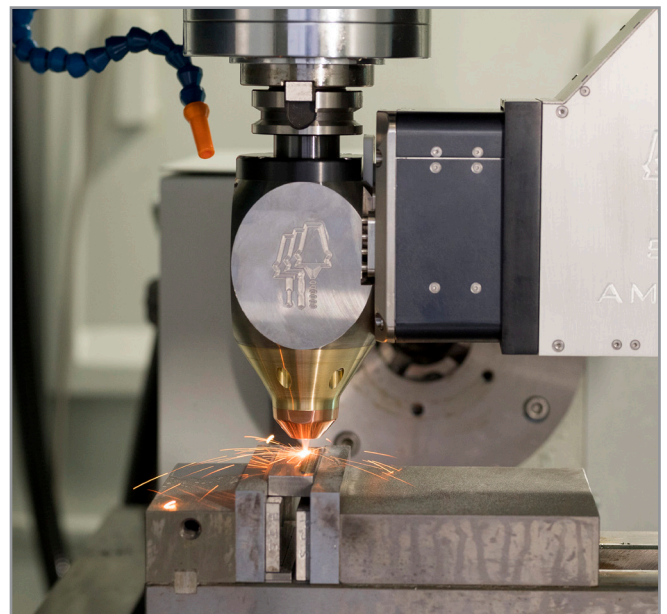
Credit: Hybrid Manufacturing Technologies. Legend: AMBIT™ FLEX 20 LMD head held in a CNC spindle depositing onto part in vice
