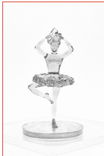
Image : 3D printed figurine produced with xolo's volumetric 3D printing technology. – Credit: xolo
