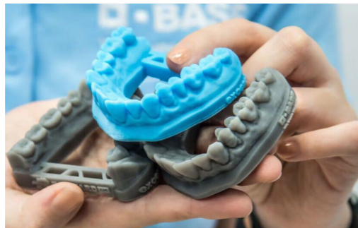
Credit: Forward AM - Dental molds produced with Ultracur3D® RG
