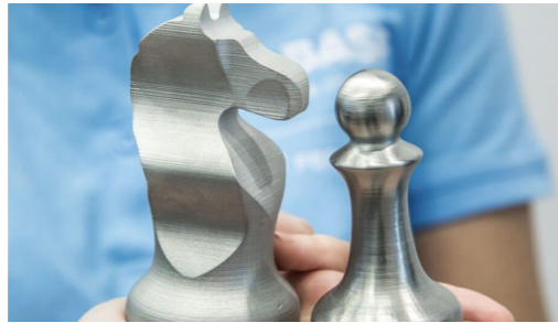
Credit: Forward AM by BASF - Part produced with a metal filament for FFF
