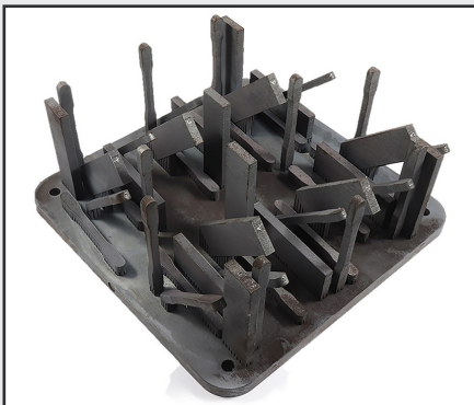
Legend: Heat treated 20MnCr5 on the build platform © GKN Powder Metallurgy
