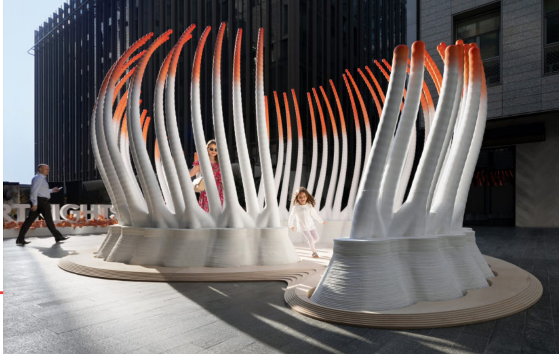
Legend: 3D Printed pavilion made from recycled plastic bottles – Credit NAARO
