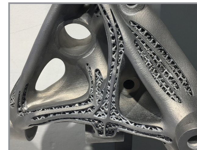
Image LEO Lane- Metallic 3D Printed support
